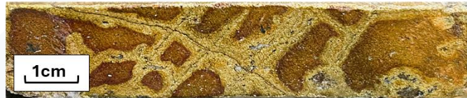
TDH01 4.6 metres at 18.54 % Cu from 57.9 metres 1 massive chalcopyrite (copper sulphide) - tarnished by length of time in core tray
