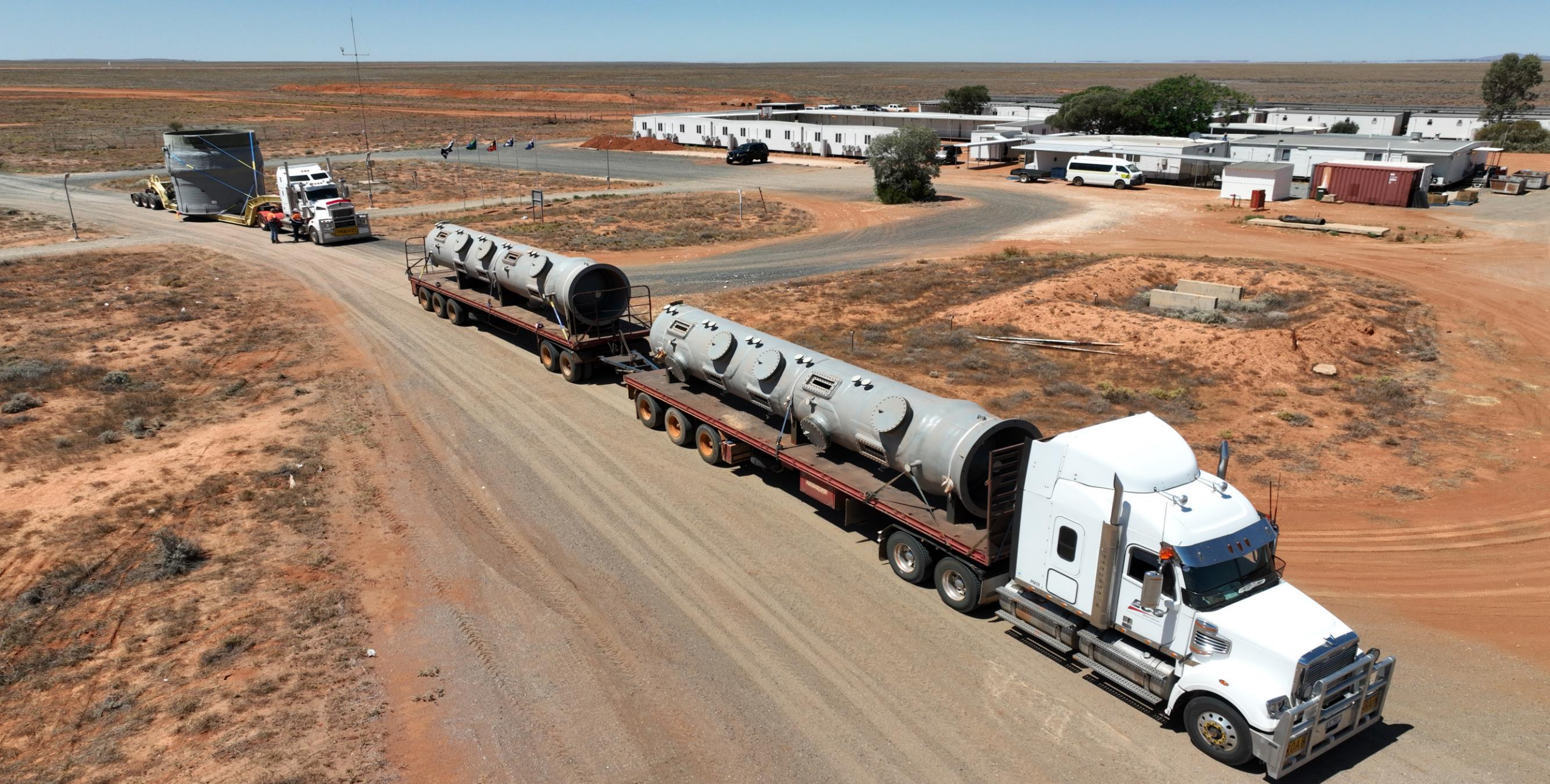
First NIMCIX elution column entering Honeymoon uranium mine site
