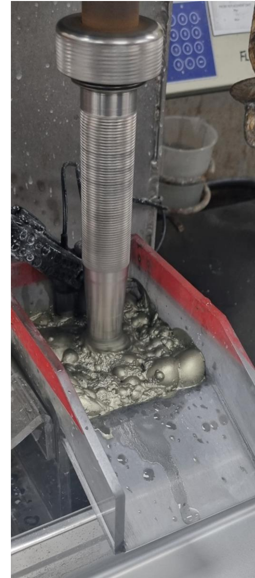
Caravel ore laboratory scale flotation testwork
