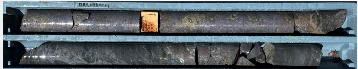
DRRCD0019 - Massive Pb-Zn Sulphides 1.7m at 26.5% Pb, 7.8% Zn, 558g/t Ag, 0.7% Cu and 0.81g/t Au from 224.5m
