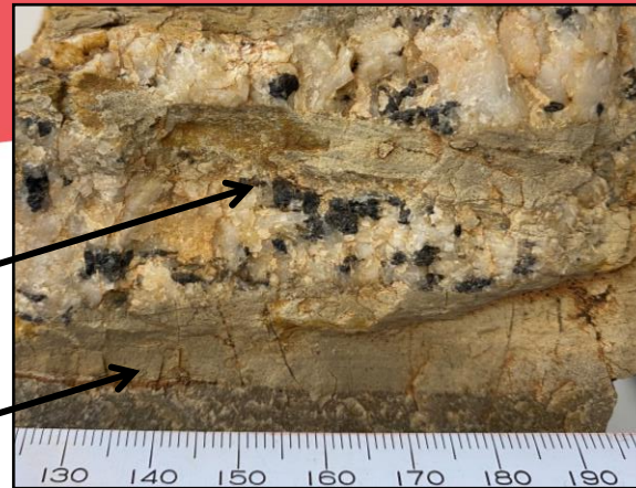
Cassiterite from Tallebung – Scale in mm
