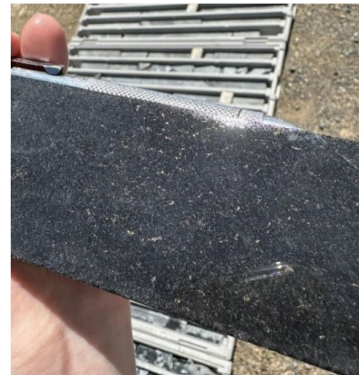
Drilling interval with Ni-Cu-Fe sulphides (within 10m at 1.2g/t PGE) 2
