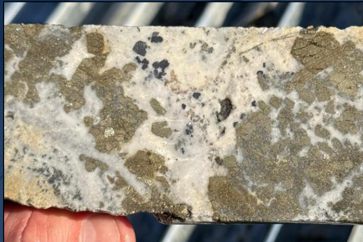
540.5 to 542.5m – 1.9g/t Au, 0.3% Cu, 1.1% Pb, 0.8% Zn and 17.3g/t Ag (3.6g/t AuEq 2 ).
