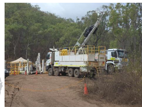
Photo: 2026 Diamond drilling at Mt Dillon target at Edinburgh Park
