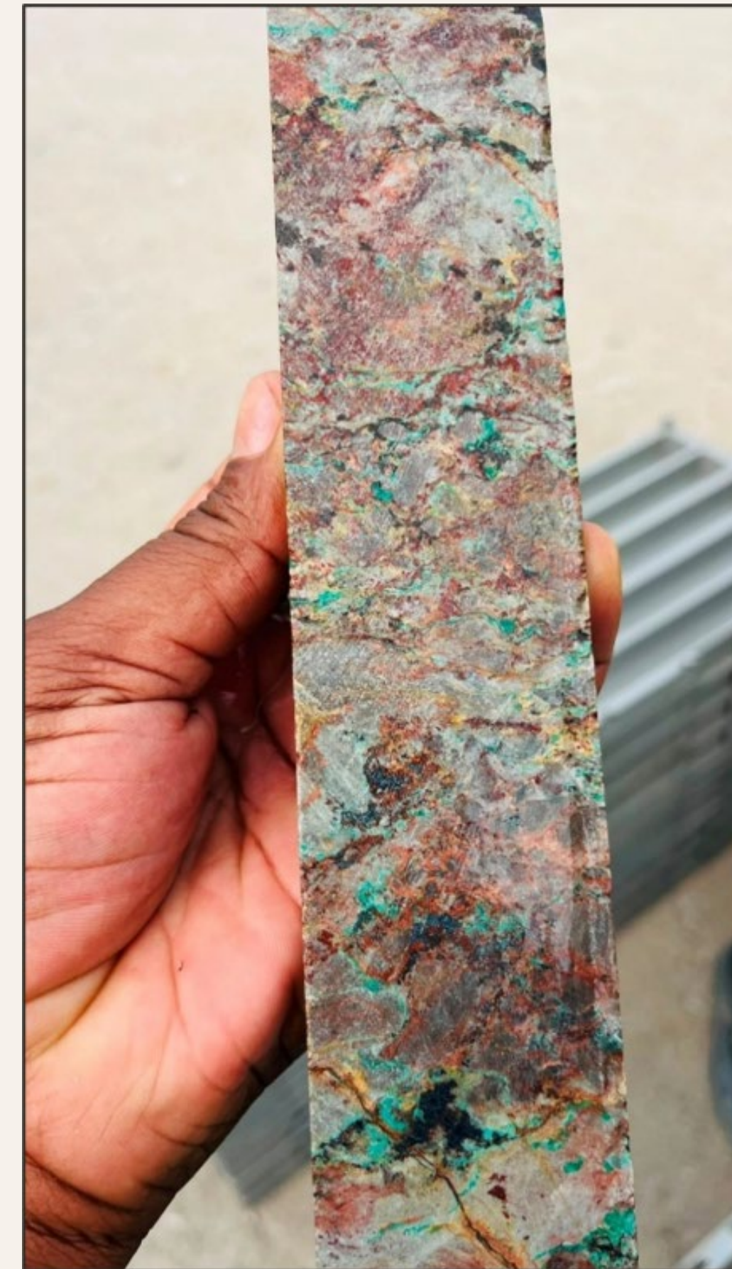
DDOT002 Core from 68.13m to 68.34m showing disseminated malachite, chrysocolla, cuprite and chalcocite mineralisation 1 (left) and DDOT001 Core from 64.03m to 64.17m showing disseminated chalcocite, cuprite and dioptase mineralisation (right).
