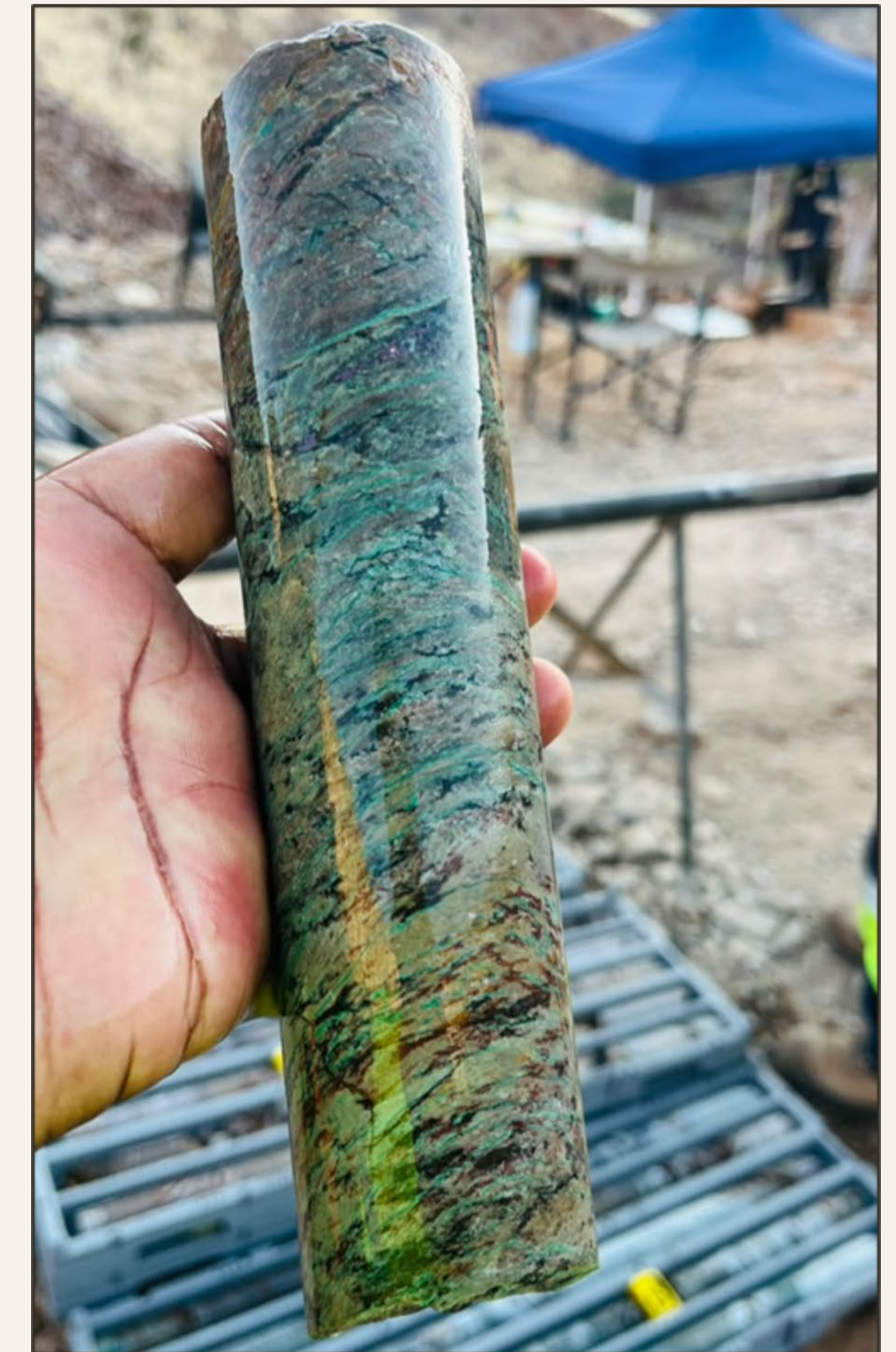
DDOT002 Core from 68.13m to 68.34m showing disseminated malachite, chrysocolla, cuprite and chalcocite mineralisation 1 (left) and DDOT001 Core from 64.03m to 64.17m showing disseminated chalcocite, cuprite and dioptase mineralisation (right).
