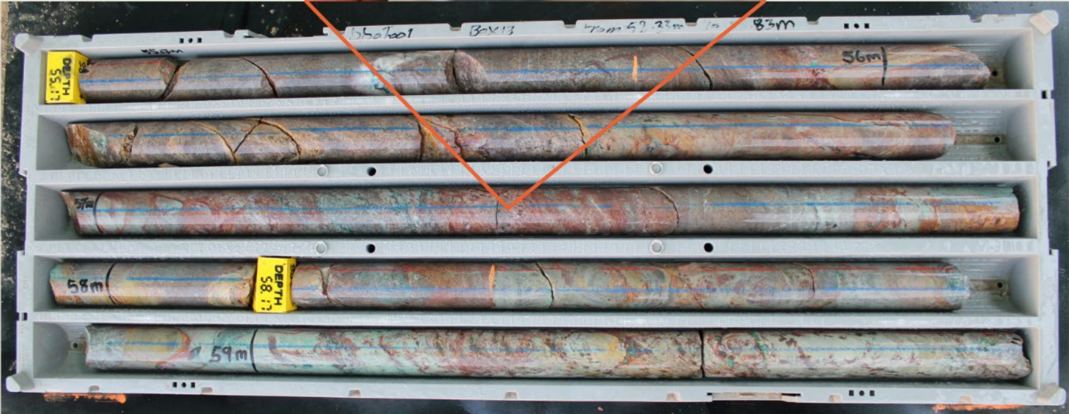
DDOT001 Core from 59.83m to 64.34m, showing a selection of mineralised drill core from ~61.17m & ~64.17m, with the visually identified copper minerals annotated 1
