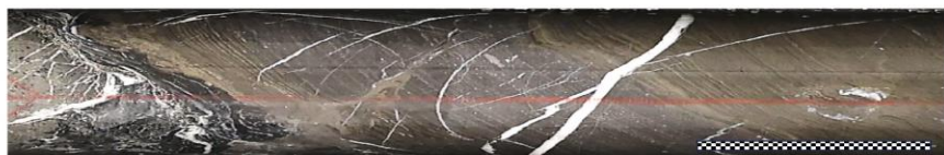
Figure 2. CD26-009 at 138.7m; altered gabbro grading into shale hosted laminated massive sulphides, predominant pyrite with brassy chalcopyrite thinly interbedded with white carbonate veins. Scale bar approx. 5cm
