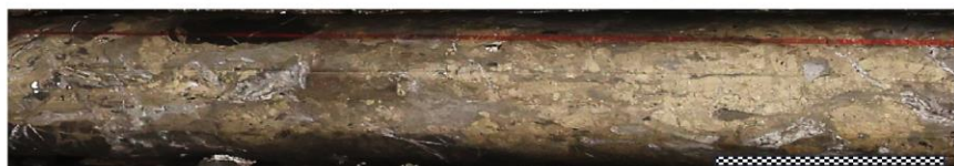
Figure 5. CD26-013 at 292.6m; Brecciated semi massive sulphides showing sulphide replacement of some clasts. The dark green sulphides are predominantly pyrite, the yellow green to brassy-yellow sulphide is chalcopyrite, with dark clasts of unmineralised shale and with white carbonate veins. Scale bar approx. 5cm
